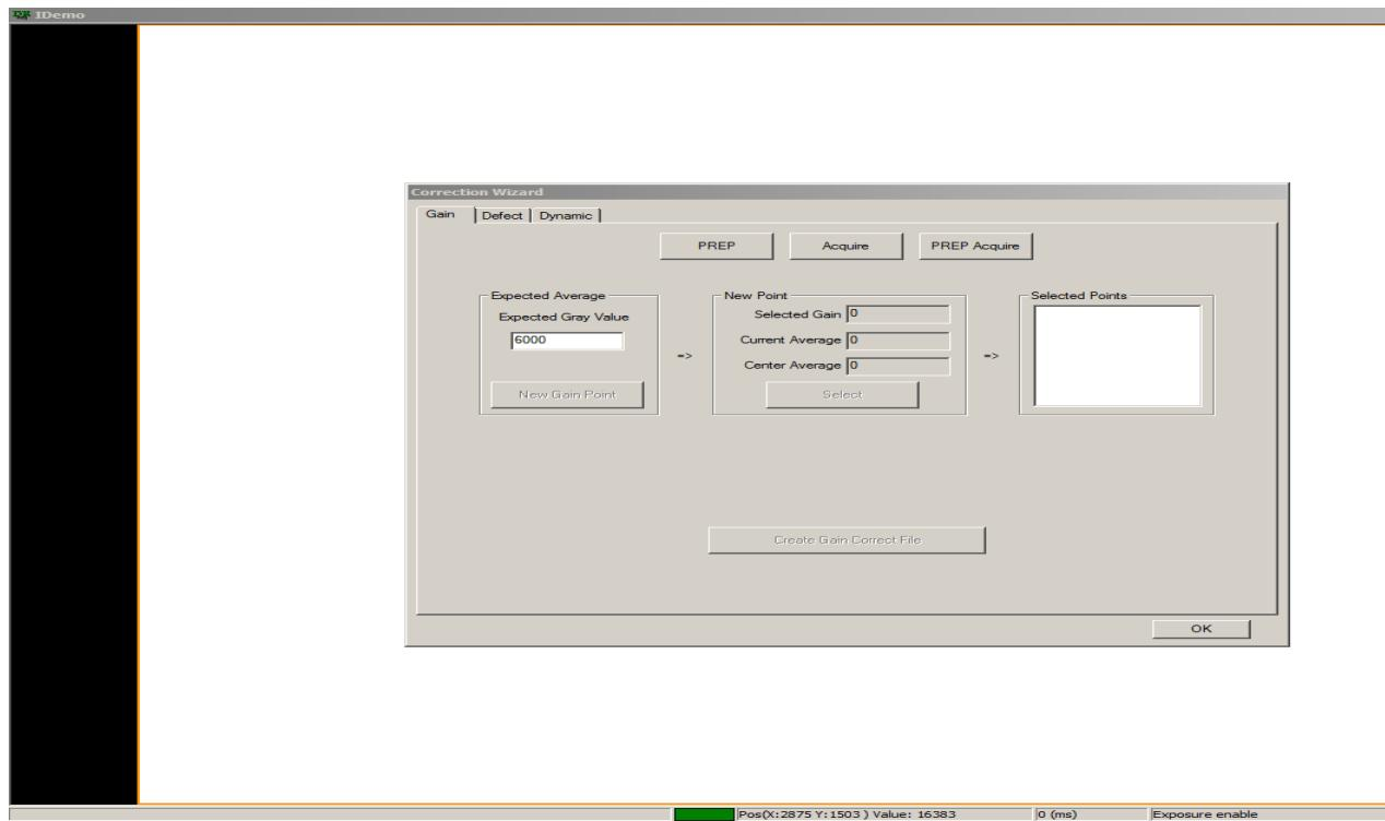
Make an exposure. The Panel activity section states the following commands image getting... (delay time:x) , exposure prohibit (post offset) , exposure enable (post offset), got image , then the center average values populates.
